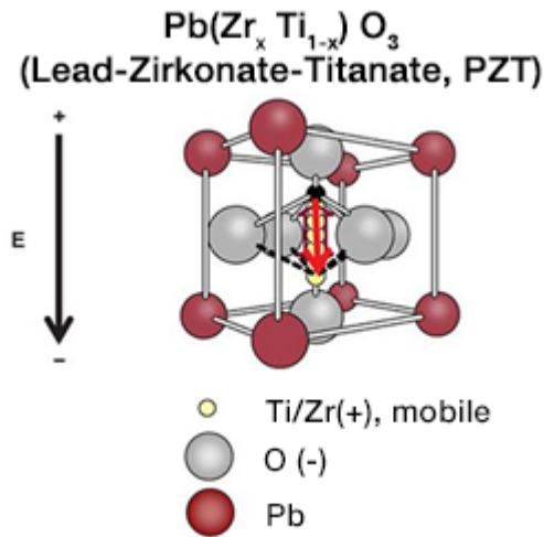
Figure 15 Structure of Lead-Zirconate-Titanate
